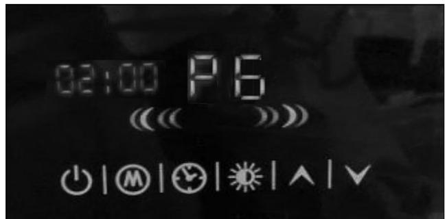
6. To power off the unit, press
